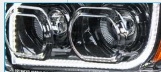
White LED position light bar changes to amber when turn signal is activated
